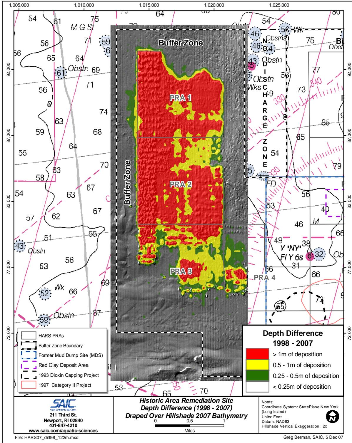
**Figure 4.2-2.** Bathymetric depth difference displaying areas of PRAs 1, 2 and 3 covered by remediation material at thicknesses exceeding 1 m (red) between the 1998 and 2007 surveys
