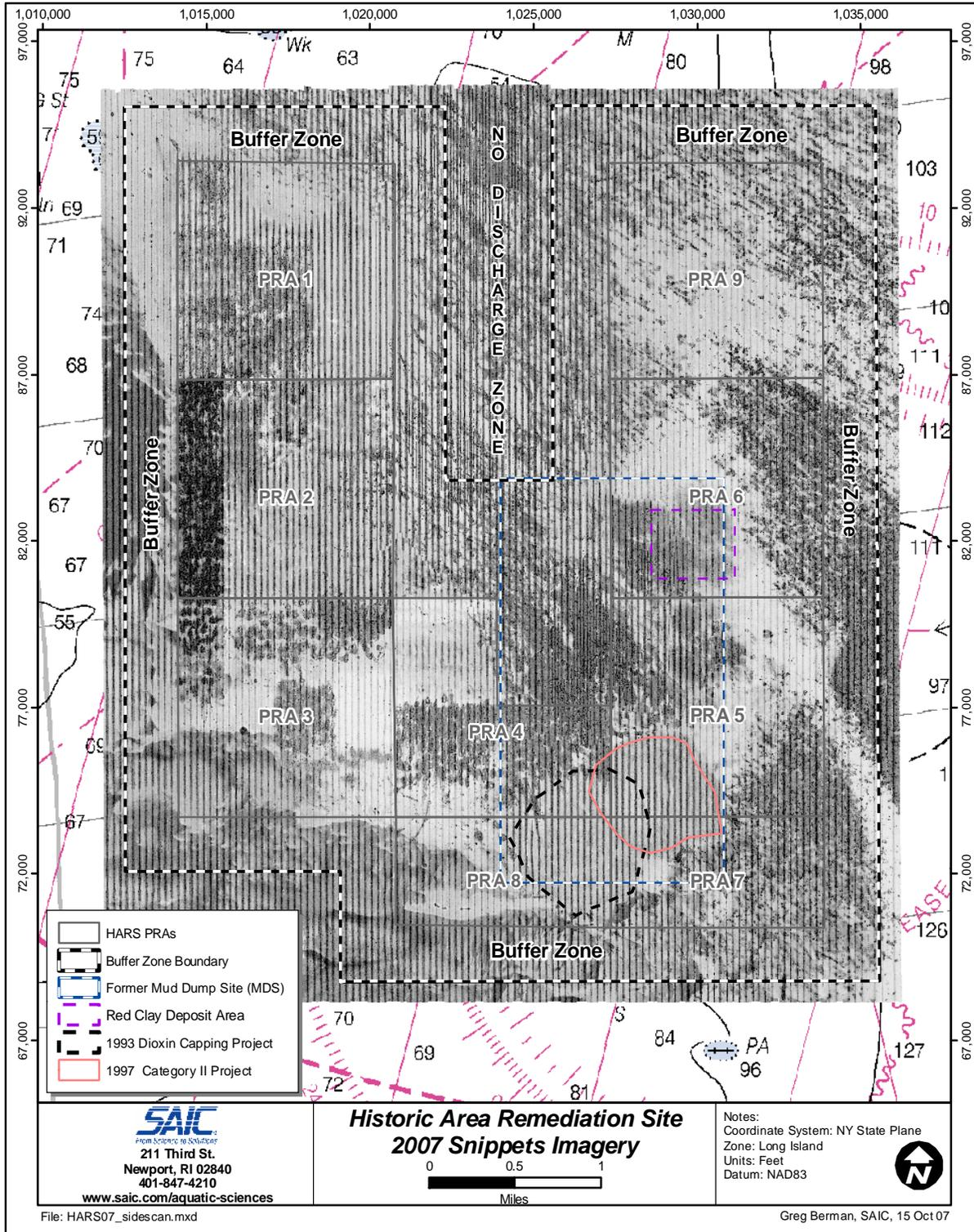
Figure 3.2-2. Multibeam backscatter imagery mosaic based on the 2007 bathymetric survey at the HARS
