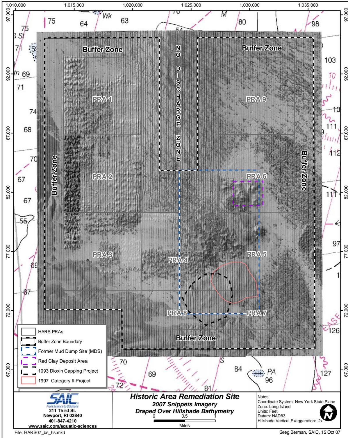
Figure 3.2-3. Multibeam backscatter imagery draped over the hill-shade multibeam bathymetry from the 2007 HARS dataset
