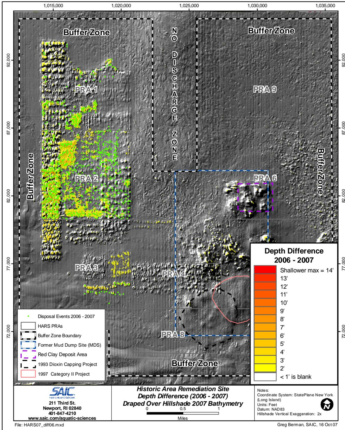
**Figure 4.1-2.** Disposal point data from the HARS from 2006 and 2007 depicted over the depth difference grid computed between multibeam surveys conducted in 2006 and 2007. The 2007 multibeam hillshade bathymetry and backscatter is included as the backdrop.
