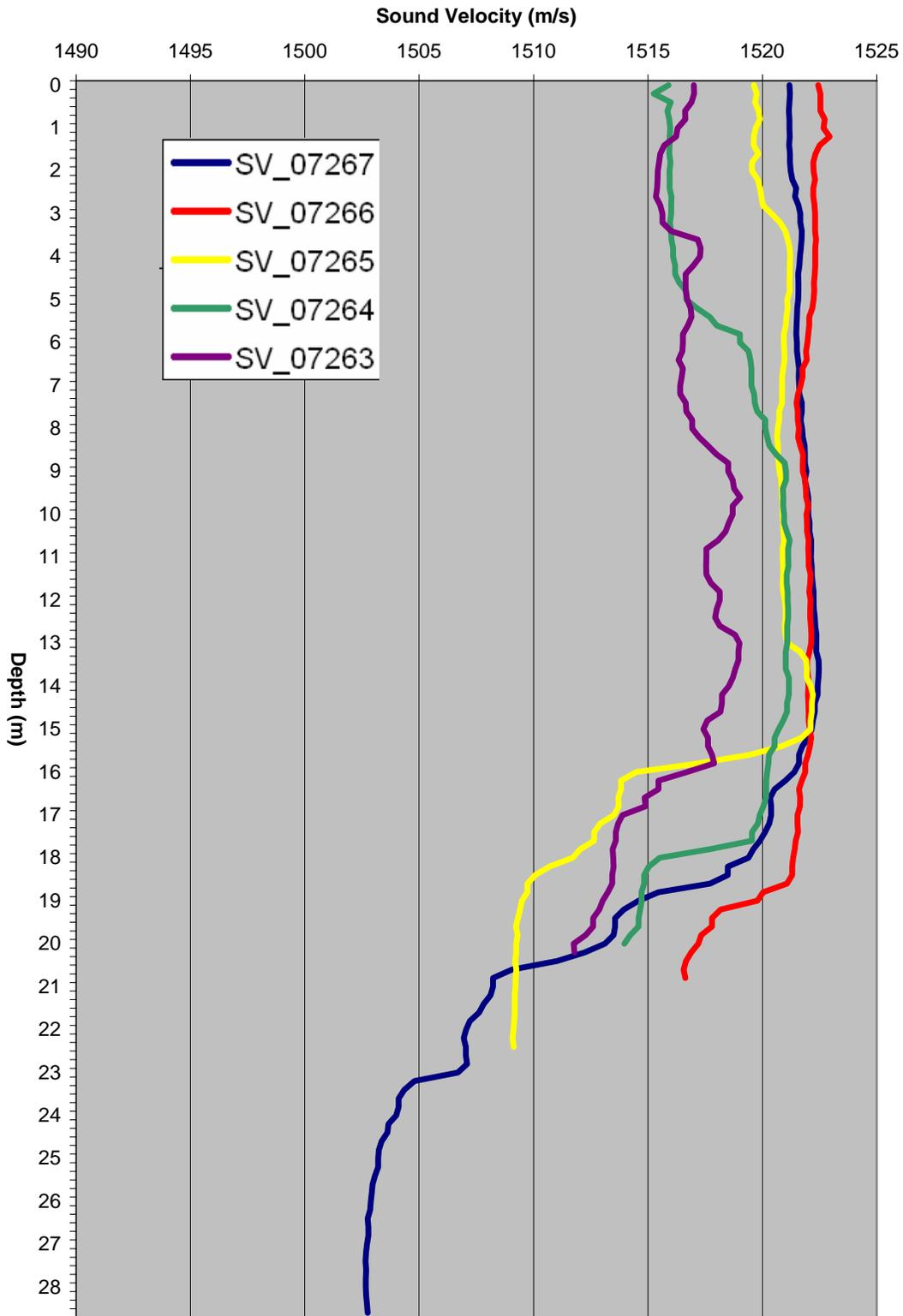
Figure 3.1-1. Sound velocity profiles representative of conditions at HARS
