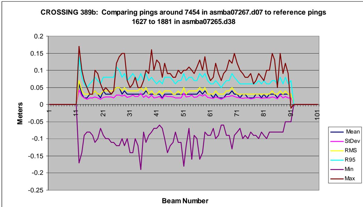
**Figure 3.1-6.** HARS Crossing 389 a/b: Beam to beam comparison between the nadir beams (reference pings) and all beams for a cross lane and a main-scheme lane in an area of overlap. Top panel uses the cross lane as the reference and the bottom panel uses the main-scheme lane as the reference.
