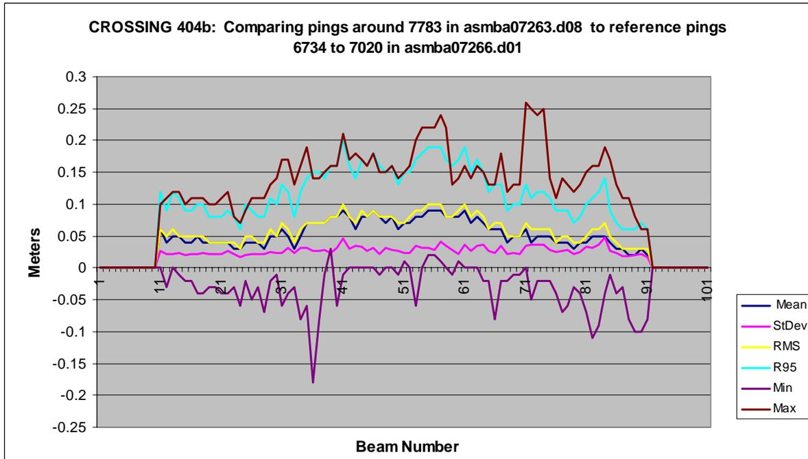
**Figure 3.1-7.** HARS Crossing 404 a/b: Beam-to-beam comparison between the nadir beams (reference pings) and all beams for a cross lane and a main-scheme lane in an area of overlap. Top panel uses the cross lane as the reference and the bottom panel uses the main-scheme lane as the reference.
