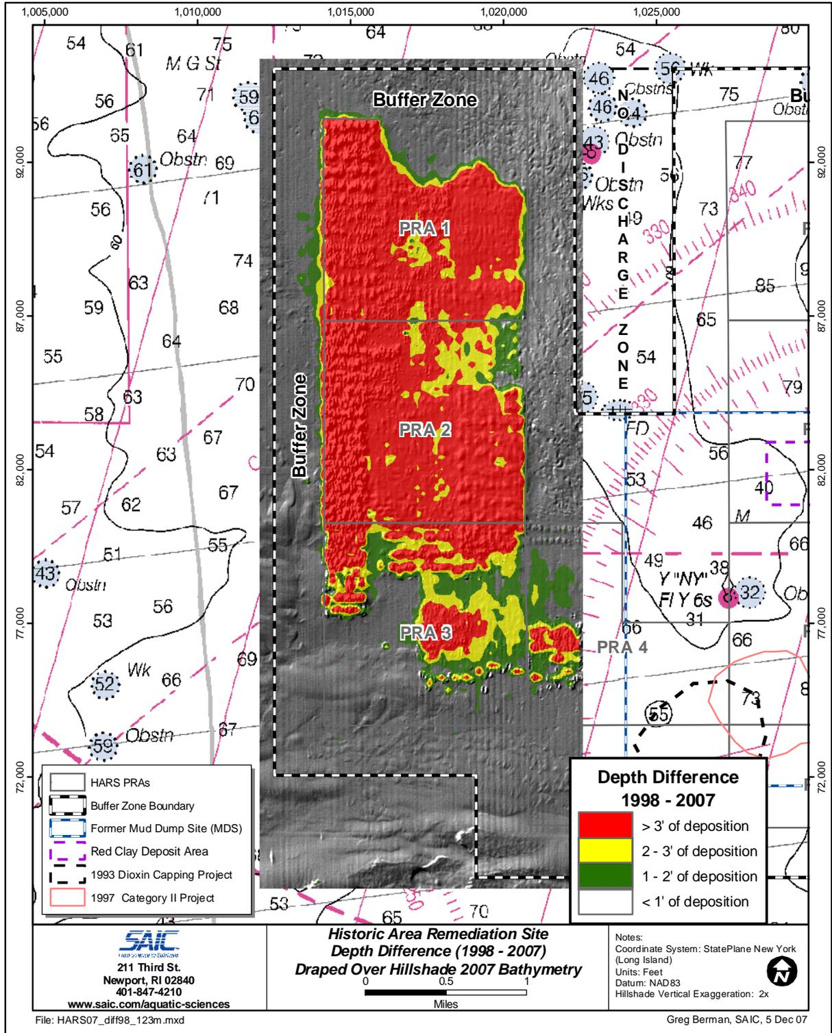
**Figure 4.2-1.** Bathymetric depth difference displaying areas of PRAs 1, 2 and 3 covered by remediation material at thicknesses exceeding 3 feet (red) between the 1998 and 2007 surveys
