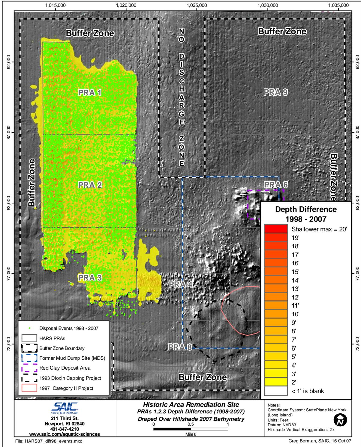
**Figure 4.1-4.** Disposal point data from the HARS from 1998 through 2007 depicted over the 1998 versus 2007 depth difference grid; the 2007 multibeam hillshade bathymetry and backscatter is included as the backdrop.
