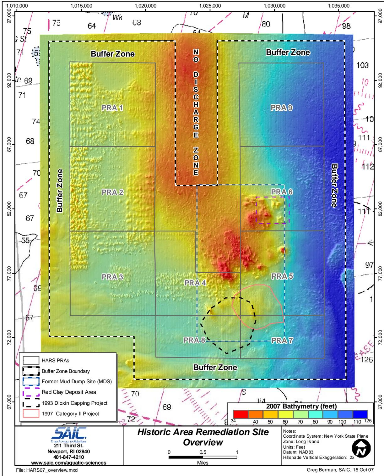
Figure 3.2-1. Hill-shaded relief model based on the 2007 multibeam bathymetric survey at the HARS
