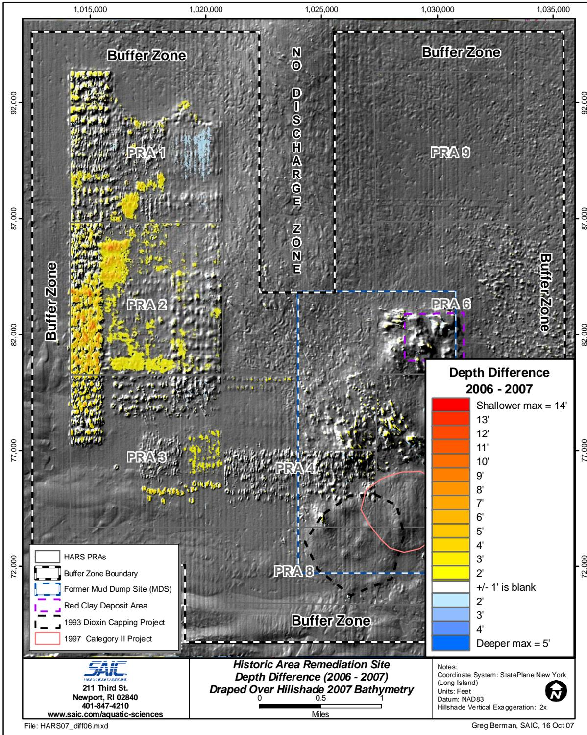
**Figure 4.1-1.** Bathymetric depth difference between the 2006 multibeam survey and the 2007 multibeam survey over the entire HARS. Yellow and red tones indicate apparent accumulation of dredged material through controlled placement, while blue tones indicate apparent consolidation or erosion.
