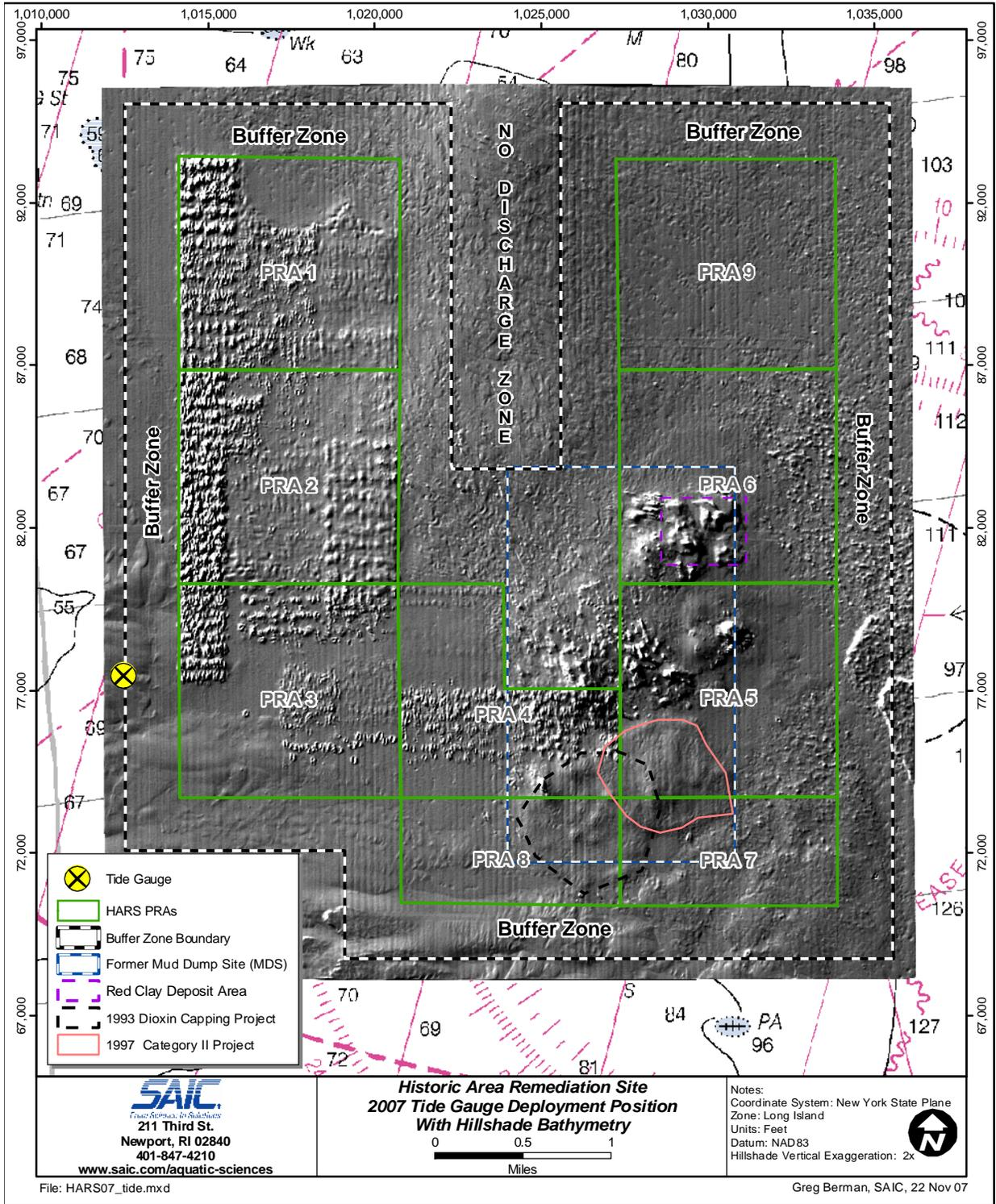
**Figure 2.1-3.** Location of the tide gauge instrument array relative to the various boundaries for HARS, the PRAs, and buffer zone. The shaded relief map of seafloor topography represents the extents of the 2007 multibeam survey area.
