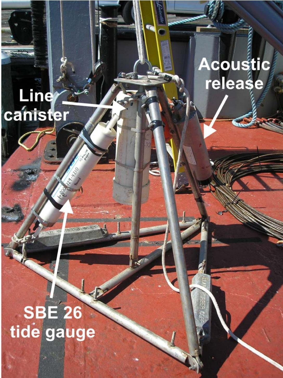
**Figure 2.1-2.** Configuration of the bottom mounted tide gauge array deployed at the HARS during the 2007 survey
