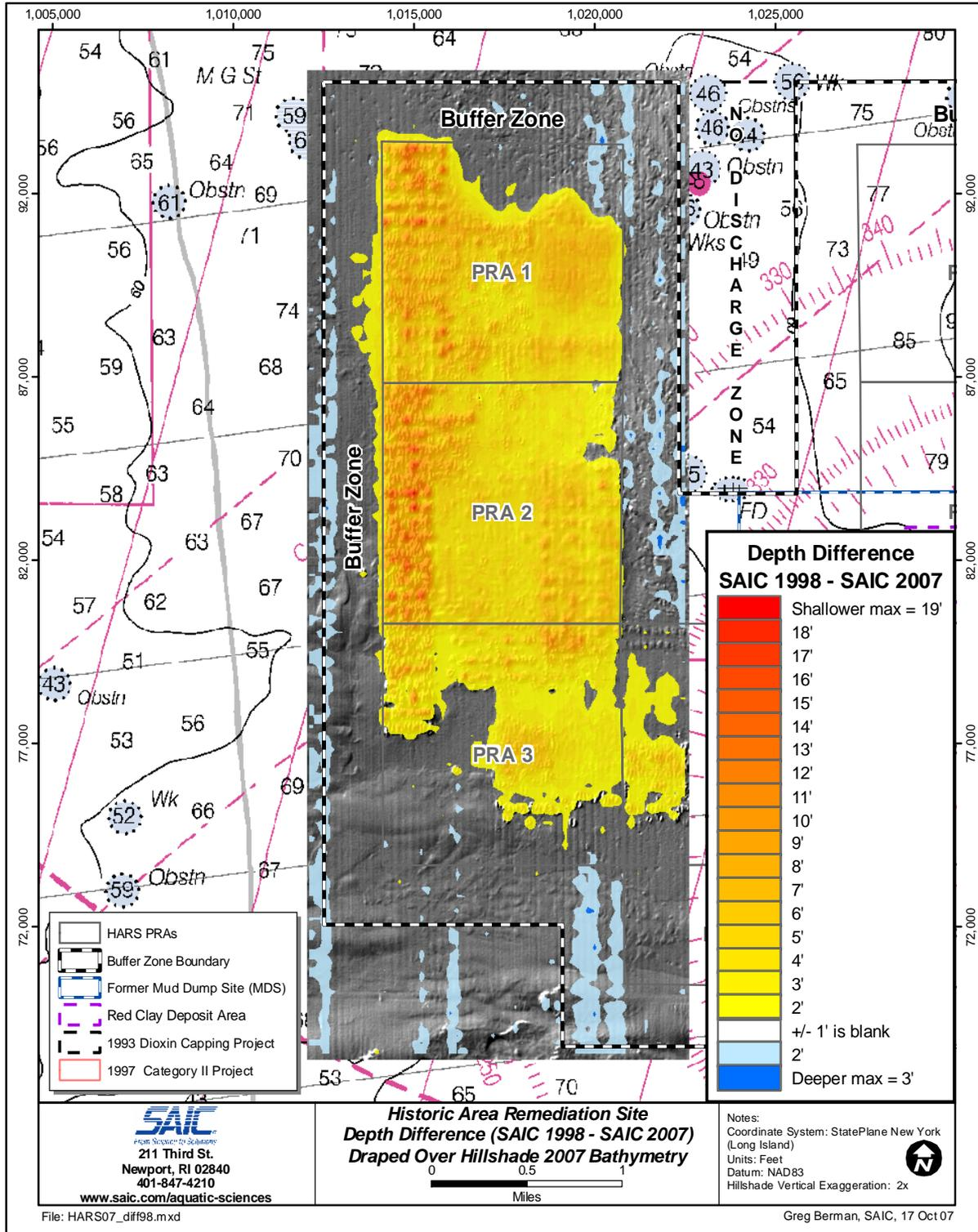
**Figure 4.1-3.** Bathymetric depth difference comparison between the 2007 multibeam and the 1998 single-beam surveys over PRAs 1, 2 and 3. Yellow and red tones indicate apparent accumulation of dredged material through controlled placement, while blue tones indicate apparent consolidation or erosion.
